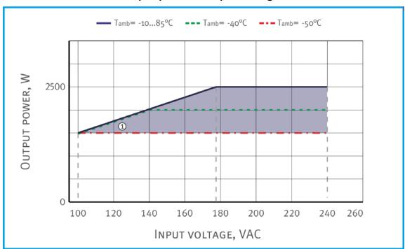
① - For ambient temperature -50°C...-10°C in gray areas of diagrams some specification parameters may not be met.
