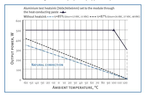
Dropping parts of the dashed and dash-dotted curves are in accordance with the **maximum temperature of the case**. Output power must not exceed the values which are limited by corresponding curve for a given ambient temperature.
