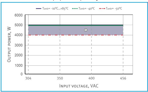
① - For ambient temperature -50°C...-40°C in gray areas of diagrams some specification parameters may not be met.
